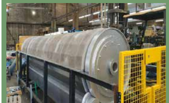
Pyrolysis boiler in production
